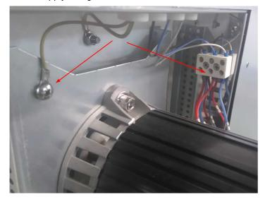
1.6. Remove the fan with its support by unscrewing the screws indicated on the following picture.
