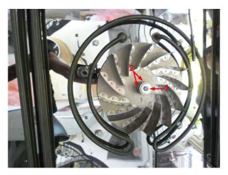
1.4. At the rear of the oven, unscrew the protective cover (12 screws).
