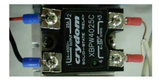
1.3. Memorize the wiring order and the positioning direction of the solid state relay.
