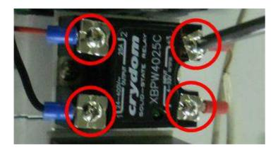
1.5. Remove the solid state relay by unscrewing if from the heat sink.
