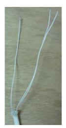
In this example, the sensing element is the alone white wire.
