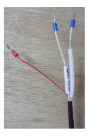
In this example, the sensing element is the red wire.
