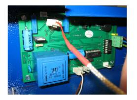
1.3. Cut the connector of the probe.
