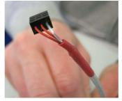
In this example, the sensing element is the white wire.
