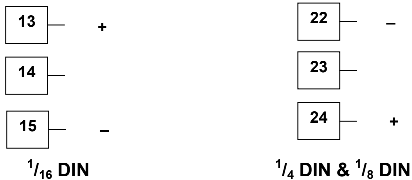
Figure 26. Option Slot 2 - Linear Voltage & mADC module
