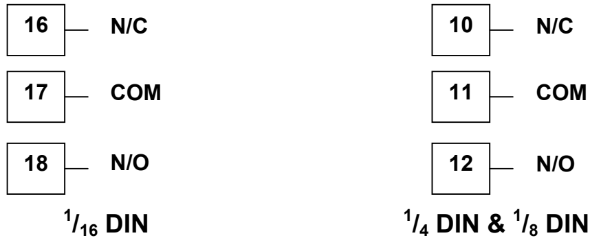
Figure 27. Option Slot 3 - Relay Module
