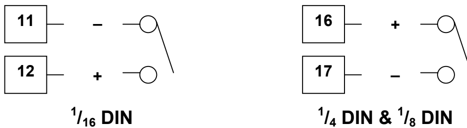
Figure 33. Option Slot A – Digital Input Module
