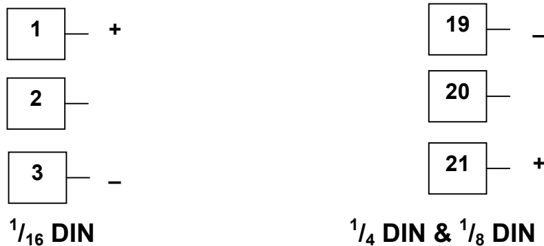
Figure 19. Option Slot 1 - SSR Driver Module
