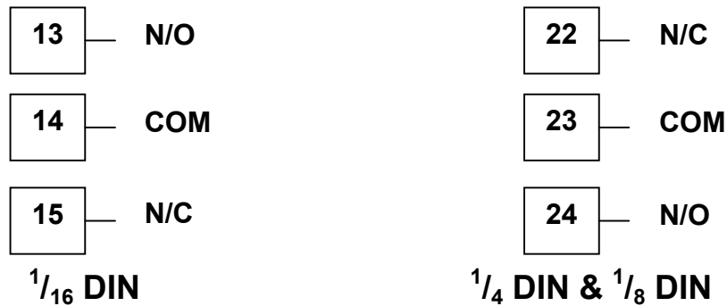
Figure 22. Option Slot 2 - Relay Module
