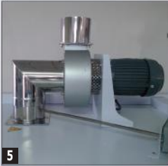
5 Air cooling extractor
